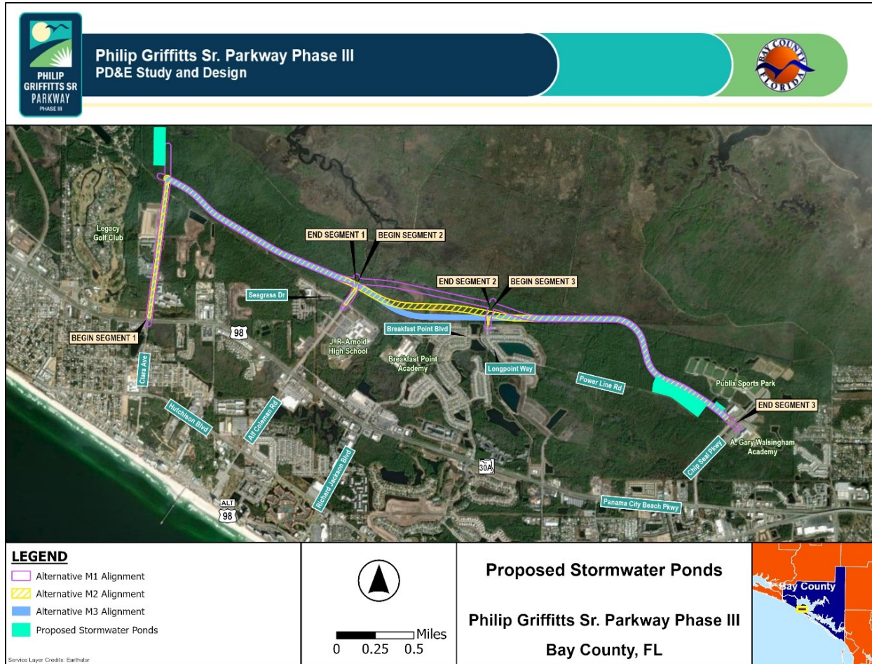
Figure C-2. Proposed Stormwater Management Facilities (Ponds)
