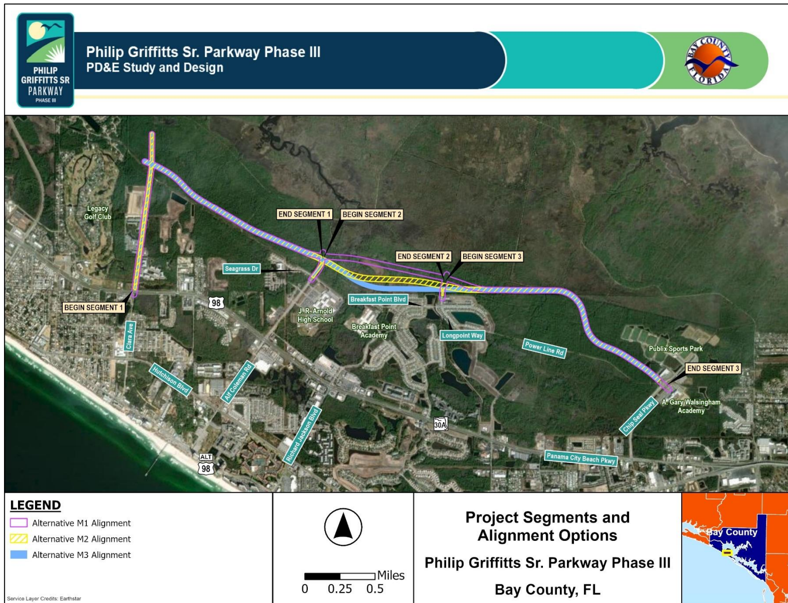
Figure 1-1. Build Alternative with Middle Segment Alignment Options
